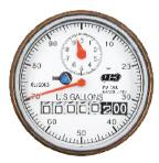
Registers include an odometer, which will give the total amount of water flow. One sweep of the hand will be equal to:
